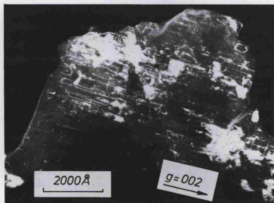
Fig. 2. Dislocations in shocked olivine from Apollo 11 (10085,26). Transmission electron micrograph. Dark field image produced by a reflection \vec{g} = 002 . Particle normal near [010]. Acceleration voltage 100 kV. (Siemens Elmiscope 101.)
